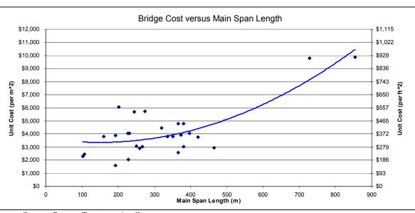
Figure S-11 Detroit River International Crossing Study Bridge Cost versus Main Span Length
